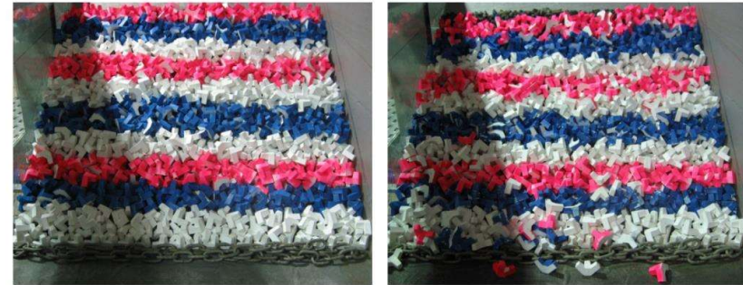
Figure 5. High-density Hanbar breakwater model with 0% damage (left), and 11% damage (right).
